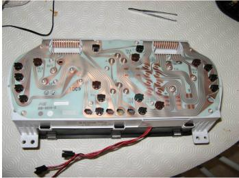
For the wires to come out, you will again need to cut a slot in the white casing and also on the black cover because they overlap. I also covered this with tape to avoid dust getting in.
