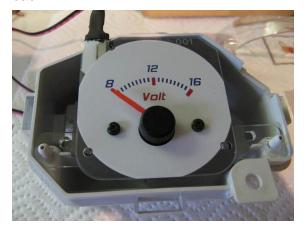
The guide says to feed the wires through but I couldn't find anywhere safe to feed them without bending too much and probably breaking the connection. As it sits on the white casing I cut a little gap on the black cover.
