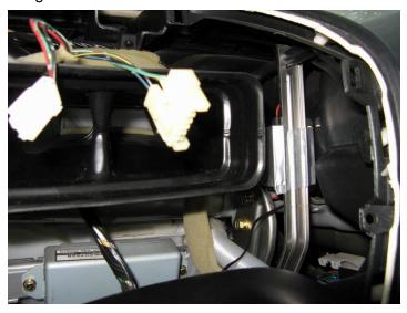
The black wire feeds through the back and connects to the bolt you see in the middle, for earth. I bought a fuse holder that came with red cable on both ends, so one end was connected to the red wire from the inverter with the black wire strip terminal:
