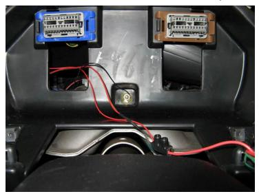
The other end was connected to the black/green wire on the foglight switch connector block. We found that it wasn't necessary to tap on this wire, we just slipped it in together with the black/green wire to test. Don't secure it just yet!!
