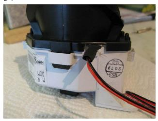
Refit everything back. I put a tape to seal the hole at the back of the clock to avoid dust.
